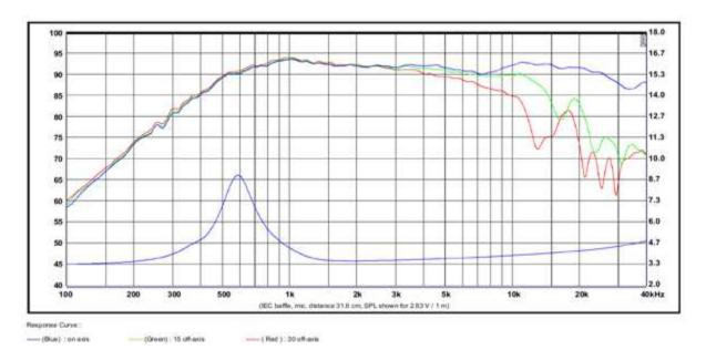
Here is my measured quasi-anechoic minimum phase response of the tweeter on my "infinite" baffle:
