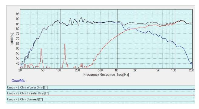
**For those that are interested, here are the actual filter transfer functions.** The early initial roll-off of the woofer's filter is for the purpose of compensating for the baffle diffraction step. The measured response shows how well this simple curve flattens the response:
