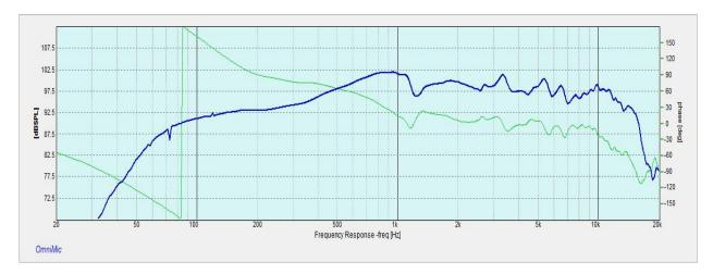
The notch in the woofer's response at 1200 Hz is real. It is most likely due to the cone's edge resonance where it terminates to the soft rubber surround. In my opinion though it is not an issue to be concerned with, as narrow band notches are generally inaudible, and I have never noticed anything in my listening sessions that I would attribute as an issue in this frequency range.
