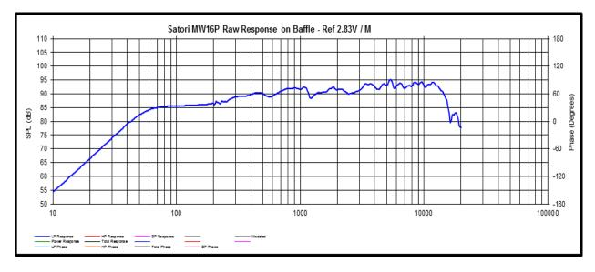
I measure the exceptional bandwidth of the driver too; the only other real difference between my measurement and the SBA graph is that my measurement shows the baffle step and hump associated with the driver being measured on my  $9^{\circ}$  x  $16^{\circ}$  baffle. This chart shows  $1/48^{th}$  octave smoothing.
