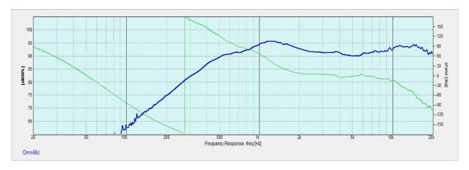
Part of the hump at 1200Hz is due to baffle diffraction in my set-up, so you need to ignore some of that, and even though my scale is compressed a bit from SB's, the two curves match up very well.
