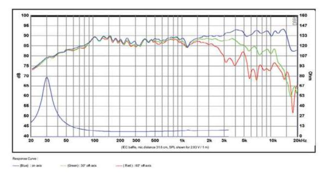
You will note the extremely wide and extended bandwidth of the driver. The notch at 1200 Hz I will comment on in a moment.
