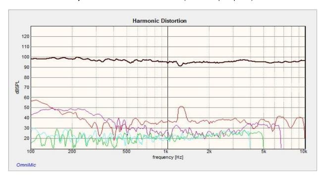
As you can see, nonlinear distortion remains quite low. The woofer's edge resonance creates, not just the dip in the response at 1200 Hz, but also a narrow peak in second order harmonic distortion. However, this peak is still low in level and fairly benign and second order distortion is fairly unobjectionable to begin with. The distortion that causes most audible issues are third order harmonics, and those remain low, at 0.1% or less THD over most of the spectrum from 300 Hz up.
