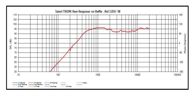
The broad hump centered at 1 kHz is due to baffle diffraction, but this is very easy to accommodate in the crossover design. As you can see, this tweeter has strong output down to 500 Hz, and relatively high sensitivity.
