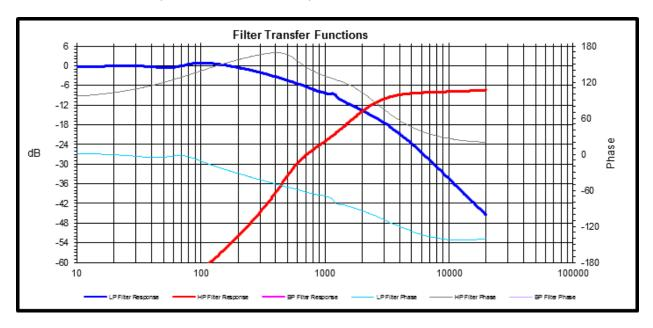
So how did the system phase response turn out? Remember this is a system with asymmetrical crossover slopes and ultimately a fourth order slope on the tweeter with it using a low Q second order electrical filter to achieve this.
