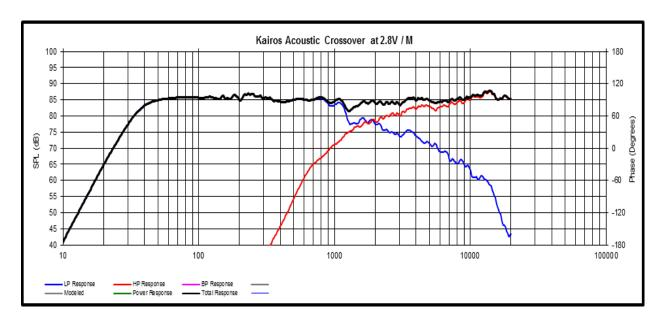
I do not have measurements along the vertical axis captured, but due to the time aligned nature of the speaker the primary lobe is straight forward on the speaker's main axis. The main design axis, by the way, was with the mic positioned between the woofer and tweeter. The nulls of the lobing are properly aimed at angles that point to the ceiling and floor. The sitting to standing test results in very little audible change in the speaker's response, which was one of my primary goals.
