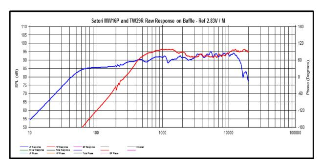
The graph above shows the raw frequency response of both the woofer and tweeter measured under identical conditions on a 9" x 16" baffle. This demonstrates the broad overlap in their frequency response. Based on this overlap and the linear, low distortion behavior of the drivers I opted to design a speaker that is time and phase accurate as well as one that has flat extended frequency response.
