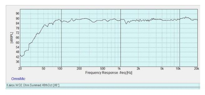
Here's a plot of the actual measured acoustic crossover. As you can see, it matches the plot above perfectly. The data in this graph is good to about 300-400Hz, below that the room begins to take over. This can be seen in the graph, but its purpose is intended to show the actual measured acoustic crossover response and summation of the drivers:
